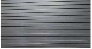
The roller shutter is made of double-skinned horizontal slats, which are interconnected by a special locks. The slats are filled with mineral wool. The roller shutter moves in guide rails and is winded onto a shaft. The roll is mounted on bearing brackets. The roller shutter achieves a speed of 0.15 m/s. Standard roller shutter is made of galvanized sheet. On customer request it is possible to be delivered with surface treatment according to RAL.
