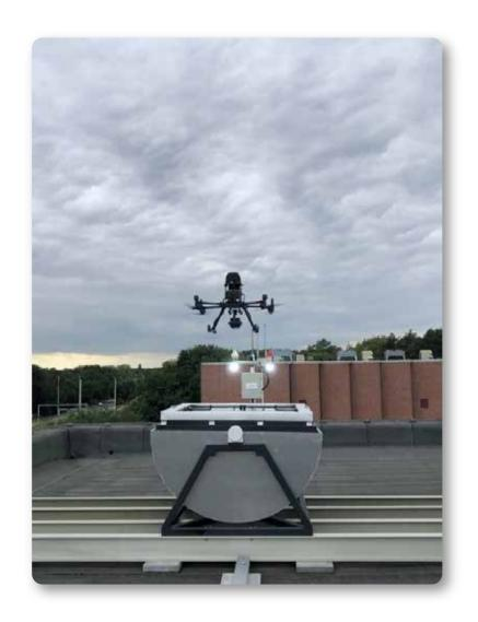
Remote operators from the ROC can remotely manage, monitor and control the drone and docking station using the FlytNow-powered software. The systems are integrated with the emergency dispatch services systems so the remote operator instantly has all information on relevant their screen when Safety Drone is called upon. The live HD-video feed and high-resolution
