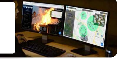
The dashboard offers live telemetry and visual data from all connected drones, with dual control from both the RC and the web dashboard. This allows for coordinated drone operations where data from multiple drones can be stitched together and shared for better situational awareness.
