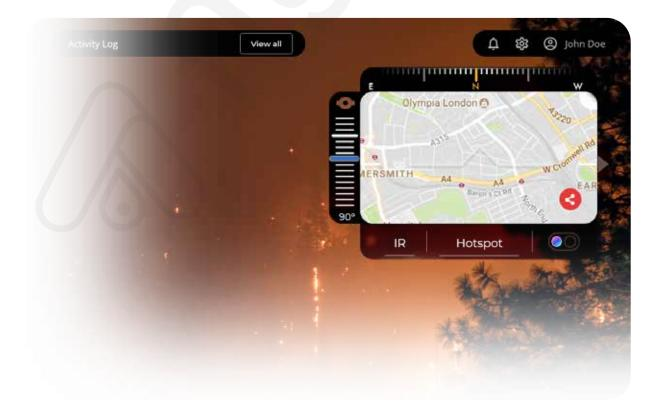
A viewer can switch between 'normal' view (RBG) and 'thermal' view (IR) if the drone is equipped with an IR sensor. In the case of DJI Mavic 2 Enterprise Dual and DJI M210 V2 Dual, the FlytNow dashboard provides the MSX view that shows the lines and edges, along with the contrast, to differentiate between regions with different temperatures.
