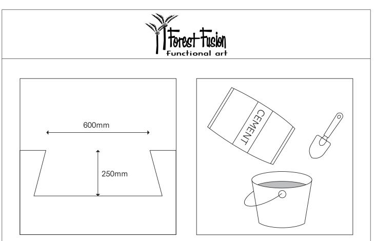
Dig a hole with a large spade 250mm deep and 600mm in diameter. We recommend digging the hole in a slight bell shape, as shown in diagram.
