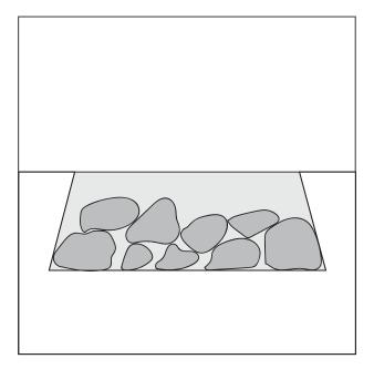
Fill hole with concrete. You may chose to add some rocks at the bottom to save on concrete.
