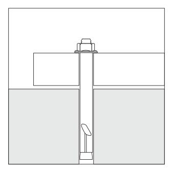
Place base back on concrete pad, lining up with the drilled holes. Insert the bolt and tighten with an adjustable spanner.
