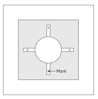
Once concrete is set, place the sculpture base on top of the concrete pad. With a pencil, mark where the four holes in the metal cross meet the concrete.
