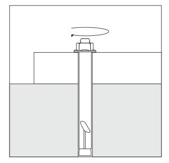
Continue tightening, allowing the sleeve to twist and pull down the base firmly into the concrete pad.
