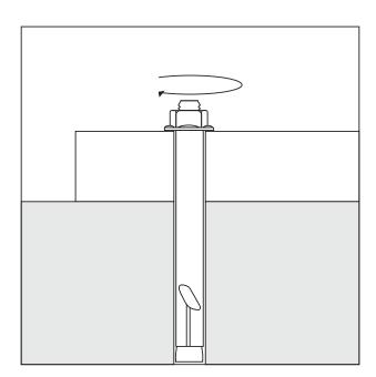
Continue tightening, allowing the sleeve to twist and pull down the base firmly into the concrete pad.
