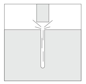
Remove debris by way of a vacuum or hand pump, compressed air, ect.
