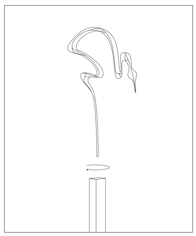
Once the base is firmly set into the ground, you can place the birds on top. You will need a step ladder for this part. Twist the bird by hand into the base until tight, the thread is about 30mm. Twist the birds into whichever position you like.
