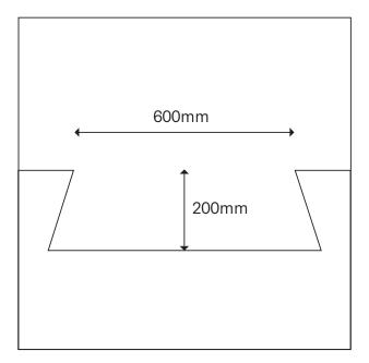
Dig a hole with a large spade 200mm deep and 600mm in diameter. We recommend digging the hole in a slight bell shape, as shown in diagram.
