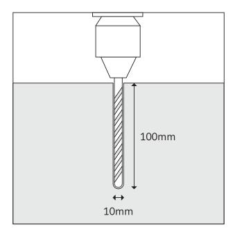
Remove the base. Drill four 10mm diameter holes, 100mm deep.
