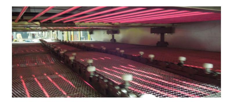
Another major advantage of infrared heaters is efficiency. Since electromagnetic radiation heating is so precise and targeted, the energy it takes to create the infrared beams transfers into the final product with little waste. The ergonomic setup of these ovens also reduces time, money, and space consumption. Other benefits of infrared heaters include:
