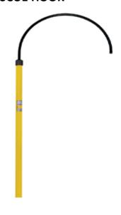
**Disconnecting stick** tube is fabricated using fibreglass. The interior of the tube is filled with thermosetting closed cell foam which is bonded with the inner wall of tube. The surface of the tube is made smooth to avoid any entrapment of external matter/impurity.
