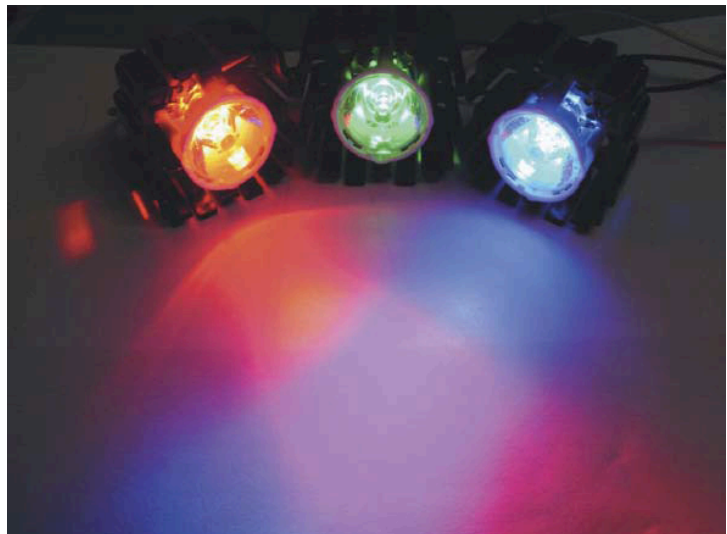
Figure 5. Three high intensity Luxeon LED lights assembled as in Figure 4 with lenses and heatsinks, and driven with identical current. Note how the simple combination of one red, one green and one blue does not give white - much more green is required. Note also how the apparent brightness of the red LED is greatest, despite the same drive current.
