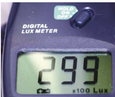
Figure 6. Digital lux meter used to measure light intensity levels. The reading shown is taken when the Helios 3000 light was operated at its highest intensity, giving 29,900 lux.
