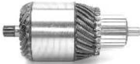
IM 2000 12 V Replacing: 132817, 74894221, 74899021 Servicing: 63114008, 63114010, 63114014, 63220030, 63220031, 63220036, 63221831, ... Slots: 25 Teeth: 11 O.D. 59,0 L. 133,5
