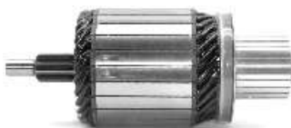
IM 3139 12 V 1.7 Kw Replacing: 231468 Servicing: M1T80081, M1T80082, M1T80381 Slots:25 Teeth:9 O.D.53,85 L.132,0
