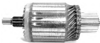
IM 3131 12 V 1.7 Kw Replacing: 235247 Servicing: M001T80481, M1T80481, PG260D, PG260F, PG260L Slots:25 Teeth:11 O.D.53,8 L.133,0
