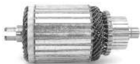
IM 305 24 V Replacing: 10626 Slots:41 O.D. 75,0 L. 193,0
