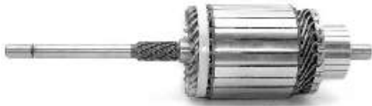
IM 493 12 V Replacing: 130241, 77771, NE034 Servicing: D8E115, D8E117, D8E129, D8E133, D8E134, D8E137, D8E139, ... Slots: 29 O.D.56,0 L. 250,0
