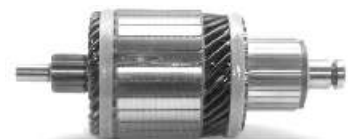
IM 3145 12 V 1.4 Kw Replacing: 1004011217, 1004011235, 238108, 5821G7, 77363235 Servicing: 0001108400, 0001108409, 0001108410, 0001122400, 0001122401, 0001122402, 0001122403 Slots:28 Teeth:11 O.D.52,0 L. 128,5
