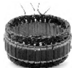
S/ 3104 24 V 50 Amps Servicing: A004TU4586, A4TU4586 Slots:36 O.D. 143,0 I.D. 113,0 H. 31,5
