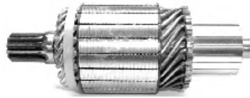
IM 3097 24 V 5.5 Kw Replacing: 132007300X0, 136517 Servicing: 03505520311, 03505520324, 03505520331, 03505520334, 03505520363, 03505520415 Slots:21 Teeth:12 O.D.65,0 L.176,5
