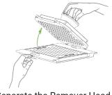
10 Separate the Remover Head from the Separator Frame by holding onto one of the clips and pulling on the round knob with the other hand
