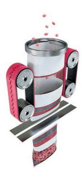
BRECOflex supplies woven endless flat belts are that are specified by many OEMs in their form-fill-seal machines. The available coatings include polyurethane, rubber and silicone with the option of having a single material or combination of materials. They feature seamless backings that provide high functional reliability with a consistent coefficient of friction and excellent wear resistance. There is no minimum order required.
