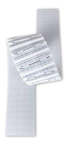
NOTE: A minimum support area of 40mm long by 80mm wide is recommended when considering a conveyed product in excess of 1kg. Recommended slider bed material is polished steel or stainless steel.
