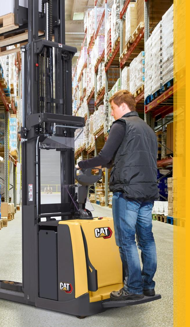
(Main picture) These stackers are precision-engineered for fast travel and fast lifting speeds that guarantee high productivity. Pedestrian and platform models lift loads up to 5.4 metres with triplex mast.
