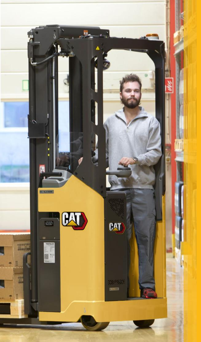
(Inset picture) Positionally adjustable controls minimise stress, strain and fatigue, while maximising precision and speed. They include an adjustable steering wheel, along with armrest-mounted features for simultaneous control of drive and hydraulic functions.
