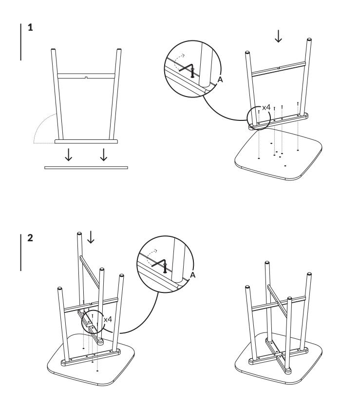
**A** - Place the feet structures on the reversed table top and lock them with the 4 screws.
