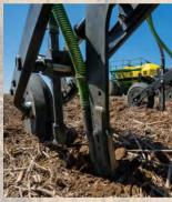
the weeds. Easily place fertilizer in dry, liquid or gas forms from 2 to 6 inches deep. Independent opener downforce can be set from 200 to 500 pounds with a trip clearance of 12 inches. The standard dry knife (shown)
