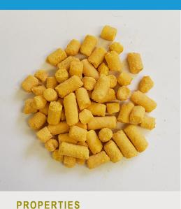
Chemical Formula  $C_4H_90CS_2K$  H-C-H  $C_4H_90CS_2K$
