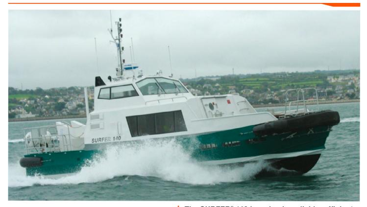
The SURFER® 140 is a simple, reliable, efficient and economical 14-metre crew boat, designed to transport passengers and lightweight equipment to oil and gas platforms.
