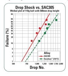
Durafuse™ LT samples in the chart (left) experienced a peak reflow temperature of 210°C and demonstrated drop shock resilience similar to that of SAC305.
