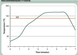
This profile is designed for use with Indalloy<sup>®</sup>282 and can serve as a general guideline in establishing a reflow profile for use with other alloys. Adjustments to this profile may be necessary based on specific process requirements.
