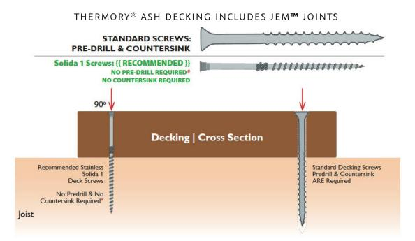
▶ Minimum screwing distance from edge: ¾". Minimum screwing distance from end: 1½". Predrilling is required, even with recommended self tapping Fixing Group Solida 1 screw, less than 8" from the end of deck board.
