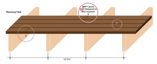
With Thermory's<sup>®</sup> exclusive JEM<sup>™</sup> Joint (joint end matched) the ends of the boards do not need to rest on the support joists. Each board must rest on and be fastened to a minimum of two joists.
