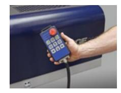
Using the control pendant, the operator can choose either forward or reverse pusher travel while the Rebel is in manual mode.
