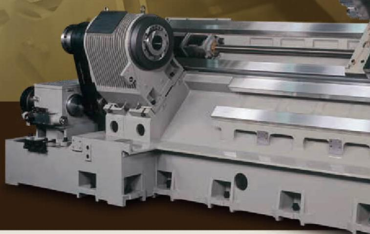
**C-axis by built-in spindle**
