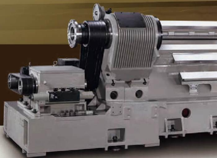
C-axis by belt-driven spindle with gearbox
