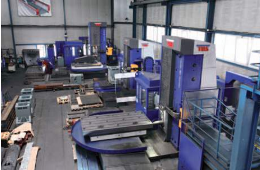
3x machine TOS Varnsdorf WHQ 15 CNC, WHQ 13 CNC, WHN 110 Q Strojirna TYC s.r.o. – Czech Republic
