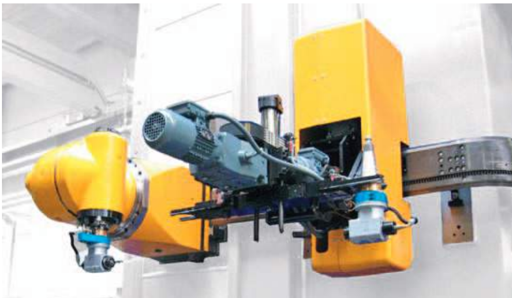
Automatic tool change to the milling head by using a four-motor tilting manipulator.
