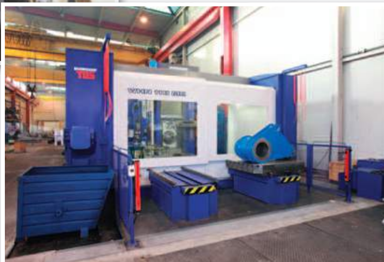
Minimisation of downtime when replacing a workpiece with a palette system that replaces a product in only 85 seconds.
