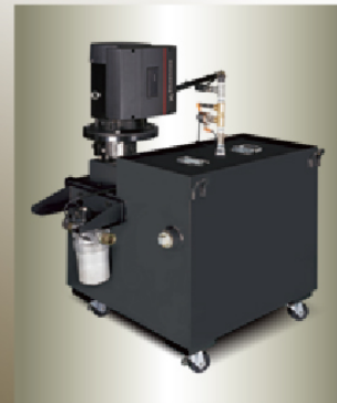
Extra CTS tank with 14~70 bar coolants and filtration system
