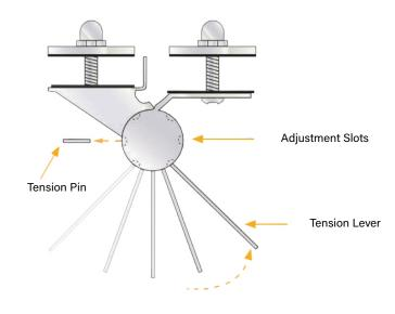
Insert tension lever tool into one of the centre adjustment slots. Gently twist anti-clockwise to untension and remove the tension Pin.
