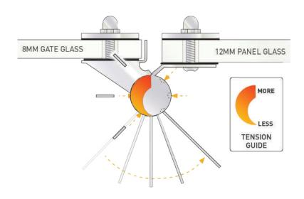
Insert tension lever tool into one of the centre adjustment slots, twist anti-clockwise and and re-insert the pin shown.
