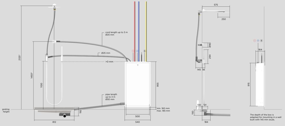
Measurements marked with \* is recommended by Orbital Systems, but still flexible. All dimensions in millimeter (mm).
