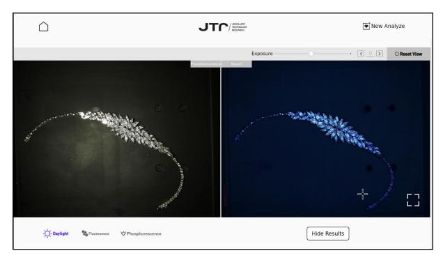
Herein, the image on the right is the result image and will not change. The result image combines both the fluorescence and phosphorescence images. However you are able to add or remove the detector red marking to the result image (in case of existence of a **lab-grown** or false positive diamond) by clicking on the show/hide result button on the bottom right corner of the screen.
