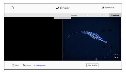
Click the square button on the bottom right corner of the result image and you will be directed to the previous screen, where you can change the amount of result sensitivity. Do not forget to click on recalculate after changing the amount of result sensitivity.
