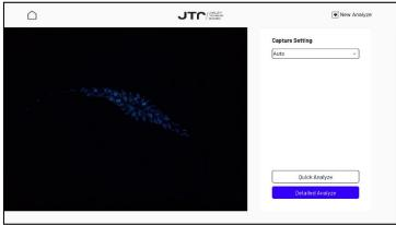
To run the test, click on your selected mode of analysis. The fan is turned off while the test is running. If quick analysis mode is selected after 15 seconds the fan is turned on and the result image appears on the screen. If detailed analysis mode is selected a screen saver with a rotating diamond crystal appears on the screen and tends to continuo while the test is running. This takes up to 4 minutes. Then the fan is turned on again and the result image appears on the screen.
