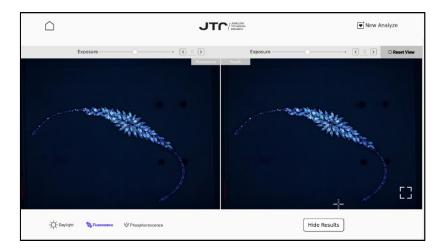
In the case of this sample bracelet since no lab-grown diamonds are present and the natural diamonds usually do not show phosphorescence no phosphorescence is shown in that image.
