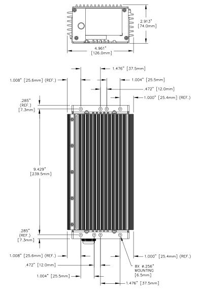
Figure 2-1: Charger Dimensions and Mounting Slot Locations
