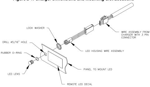
Figure 2-2: Remote LED Installation
