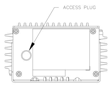
Figure 3-1: Location of the Access Plug for the Active Charge Profile DIP Switch
