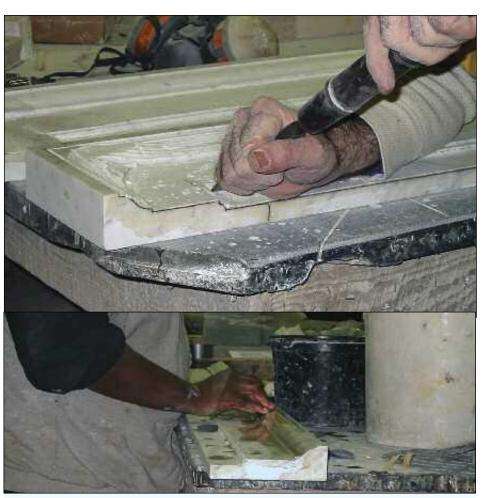
Above: A Hilgartner stonecarver uses a hydraulic chisel to prepare molding to match the door frames at the Tremont Grand. Little has changed in how such architectural stone pieces are prepared by hand, except the addition of power tools. Hilgartner is one of the few stone companies to still use an apprenticeship program to train a new generation of stone carvers.
