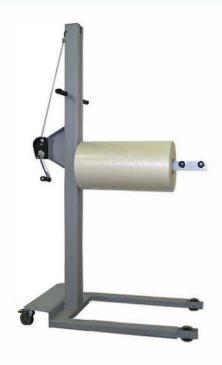
This manually operated device will lift films weighing up to 80kg and simultaneously ease the roll replacement in the machine. The loading crane works as a cable reel with a brake, thus, the roll replacement becomes a very simple operation even for a single operator.
