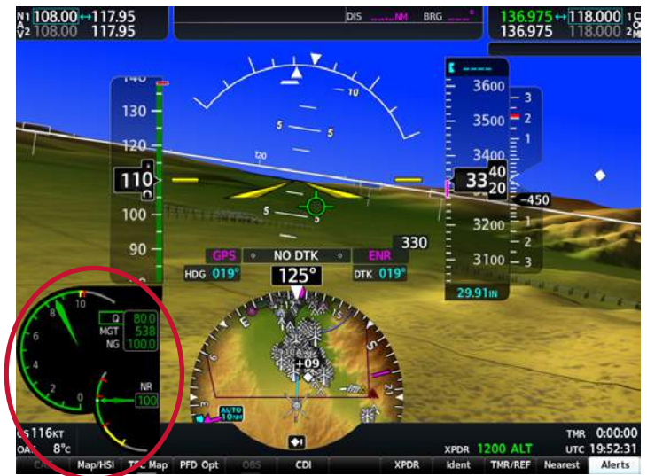
Power Situation Indicator.
