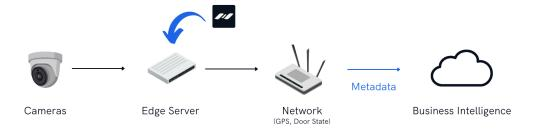
Traditional sensors used onboard vehicles often only have a single purpose as opposed to Al Video Analytics which can power a variety of use-cases from a single input type: Cameras. Leveraging the existing onboard camera infrastructure, the novel solution provides significant cost savings to operators not only during initial procurement but also when maintaining the system.
