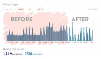
The AlertAQ water intelligence platform shows the amount of water used before and after a water cooling tower leak was fixed.
