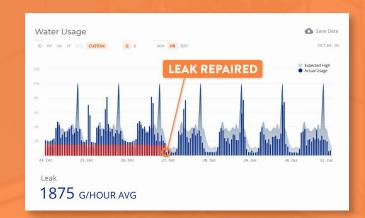
The staff used data from the AlertAQ Building Insights Dashboard such as flow rate, % of time water was running and Al-powered analytics to narrow down the cause of the leak which turned out to be a broken plumbing fixture. The leak was fixed within a few days and high water bills were averted.
