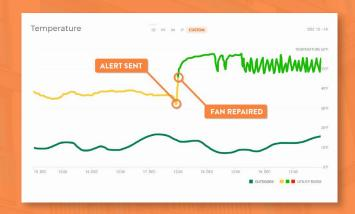
On December 15 at 11:56 a.m. the maintenance staff received a text message from an AlertAQ sensor which stated that the temperature in the utility room was 36°F and dropping.
