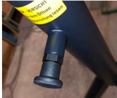
As the load increases, the support provided by the gas strut decreases! The upper part must not be twisted against the lower part when the locking pin is open! **Risk of damage and tipping!**
