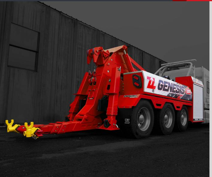
The Zacklift GENESIS 30T is a fifth-wheel, detachable, 30 TON integrated boom and under lift system. Finally, a tow system that gives the user superior flexibility with zero compromises made on capability and quality. The innovative GENESIS 30T system gives the user the ability to "Build-A-Fifthwheeler"<sup>™</sup> exactly as they need without the expense and limitations that come with standard heavy duty tow trucks.
