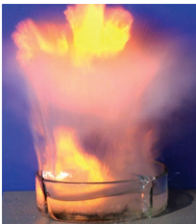
Figure 5 Explosive reaction between sodium and water
