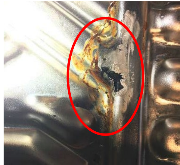
Corrosion and pitting on plate from a heat exchanger
