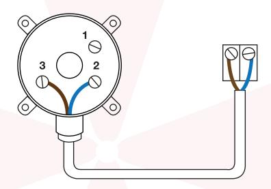
For airflow pressure switches use PCB terminals marked either intake or extract fan, these interlocks have a time delay in the software to prevent the effects of pressure switch flutter.
