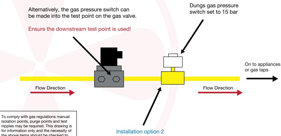
isolation points, purge points and test nipples may be required. This drawing is for information only and the necessity of the above items should be checked to ensure compliance with the current regulations.
