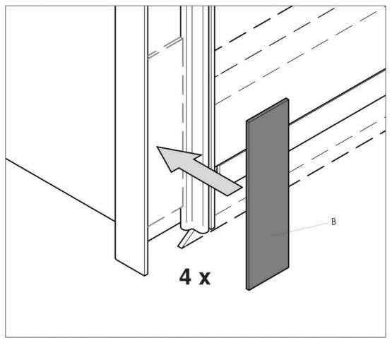
B Wear-resistance plate (Niro plate 150x90x2-1.5 mm)
