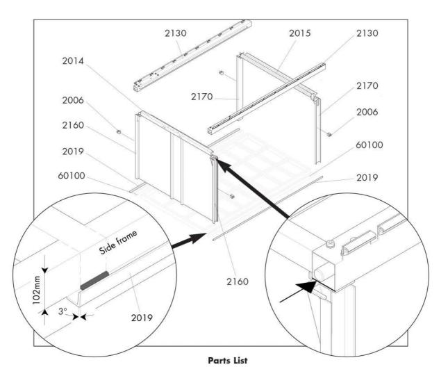
2006 Bracket for linkage (assembled)
