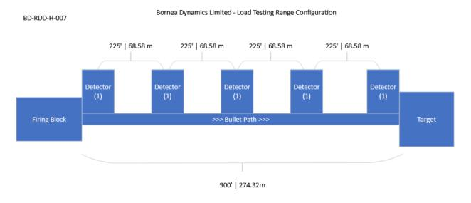
The detectors, rifle, and target were arranged as follows:
