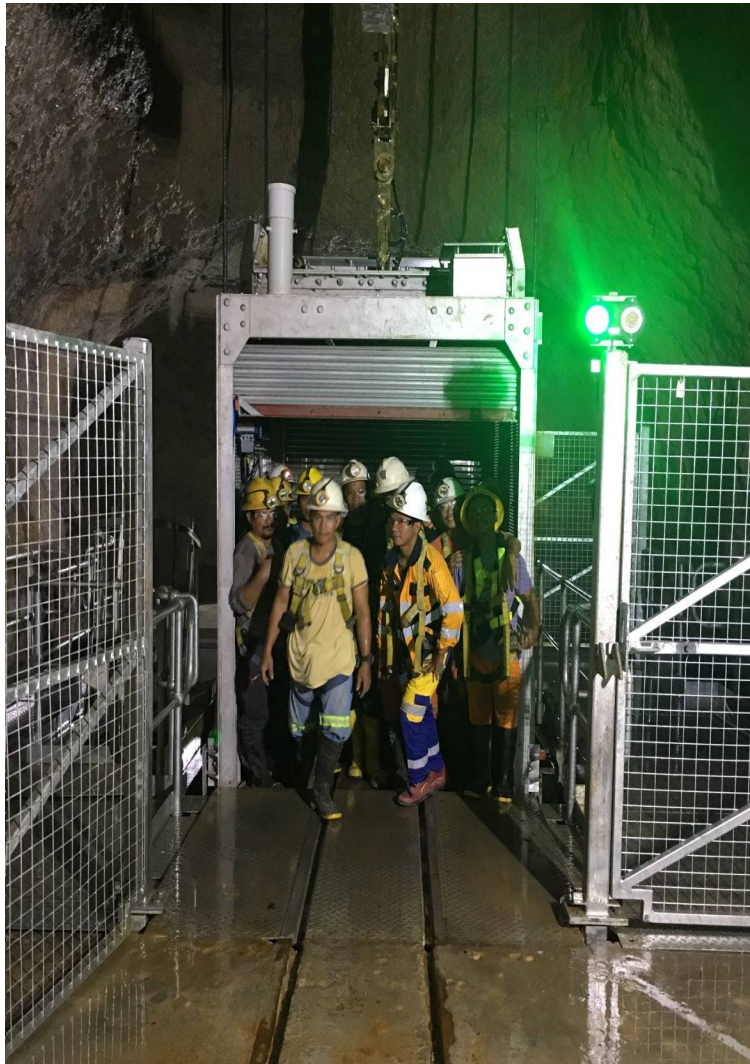
Picture 2. E15 service shaft in use: Miners disembarking on level 10
