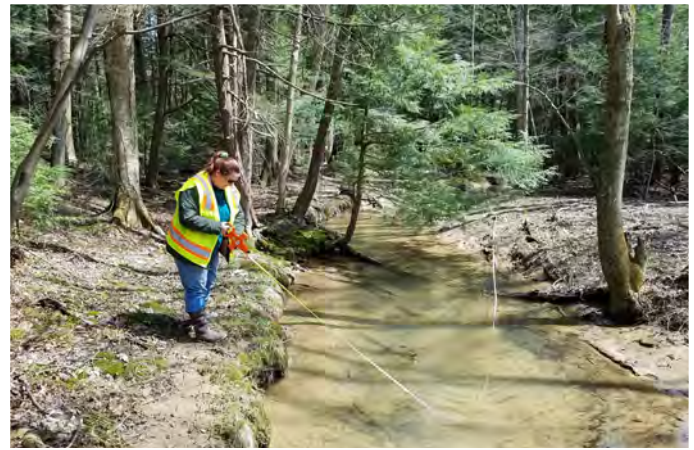
Above: District staff measure an un-impacted section of the stream to mimic in the new culvert.
