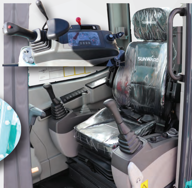
Enclosed cab offers Air Conditioning, LCD Touchscreen, and fine control features
