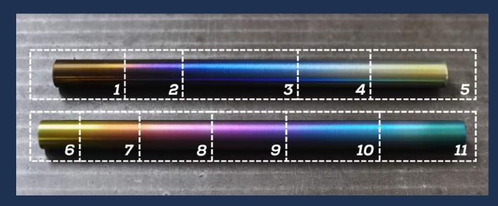
We can anodise your frame with a range of different colours although it is worth noting that the process is relatively difficult to control precisely so we ask that riders choose a colour range from the included diagram.
