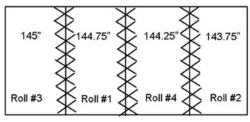
**Direct Glue:** After roll sequencing is established and carpet is dry laid, glue half of the roll with the longest pattern measurement and half of the roll with the next longest pattern measurement lengthwise. Apply seam sealer and power stretch the roll with the shorter pattern measurement to match the longer one by starting in the center of the seam and stretching towards the ends. Stay nails may be required to secure the carpet as the adhesive sets.
