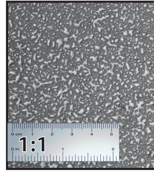
150-185 ft<sup>2</sup> (13.9-17.1 m<sup>2</sup>) Match spray pattern by placing guide on floor.
