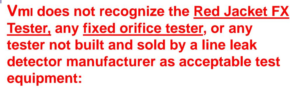
For generating catastrophic (3 GPH@10 PSI) line leaks or for being used to perform annual testing of Vaporless MLLDs or ELLDs. Reasons include:
